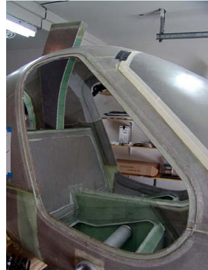
Rotor Tower dry fit - multiple mods since, including carbon reinforcement, seat belt anchors, etc. Wing Mt. Tubes aligned & attached.
