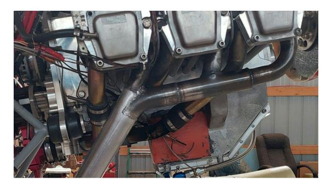
So was it worth it? I have flown 5.7 hours since the change, in temperatures from -10C to 9C. Before the change, I avoided flying in temps much below 0 because the engine ran so poorly. It now runs fine at -10C. EGT spread in cold temperatures decreases by about 70F. I am now able to run the engine leaner and it also looks like my fuel consumption is lower. It turned out to be a lot work and it took about 3 times longer than I expected but it paid off.
